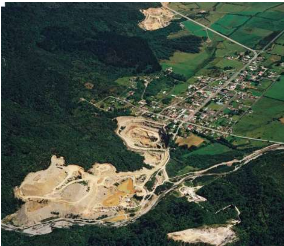
Figure 87 Jones Flat open pit gold mine (centre) in Quaternary alluvial gravels, apparently derived from Donnelly Creek (left) on the edge of Ross township. Deep leads or horizons of high gold values were worked underground beneath Ross township. The photograph was taken in 1995. Subsequently the pit was enlarged, and mining ceased in 2004. The quarry in the lower right is in limestone (GNS photos CN38487/22 and CN38488/23 composited, photographer Lloyd Homer).
