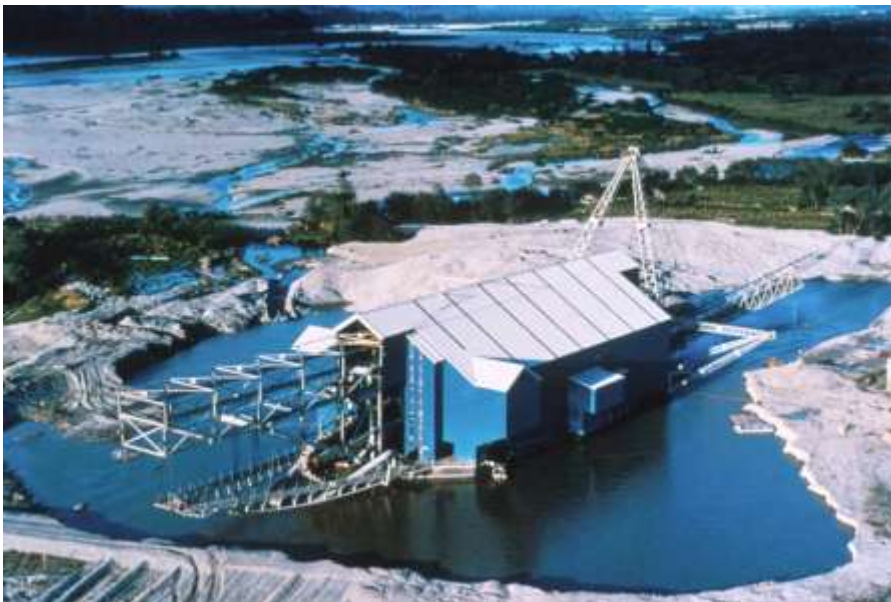
Figure 80 The Grey River gold dredge operated by Birchfield Minerals Ltd at Ngahere, with the Grey River beyond. The dredge is 150 m long from the front A frame to the end of the stacker and reaches 30 m above the water line. (Photo after Figure 1 of Cotton & Birchfield 2006).
