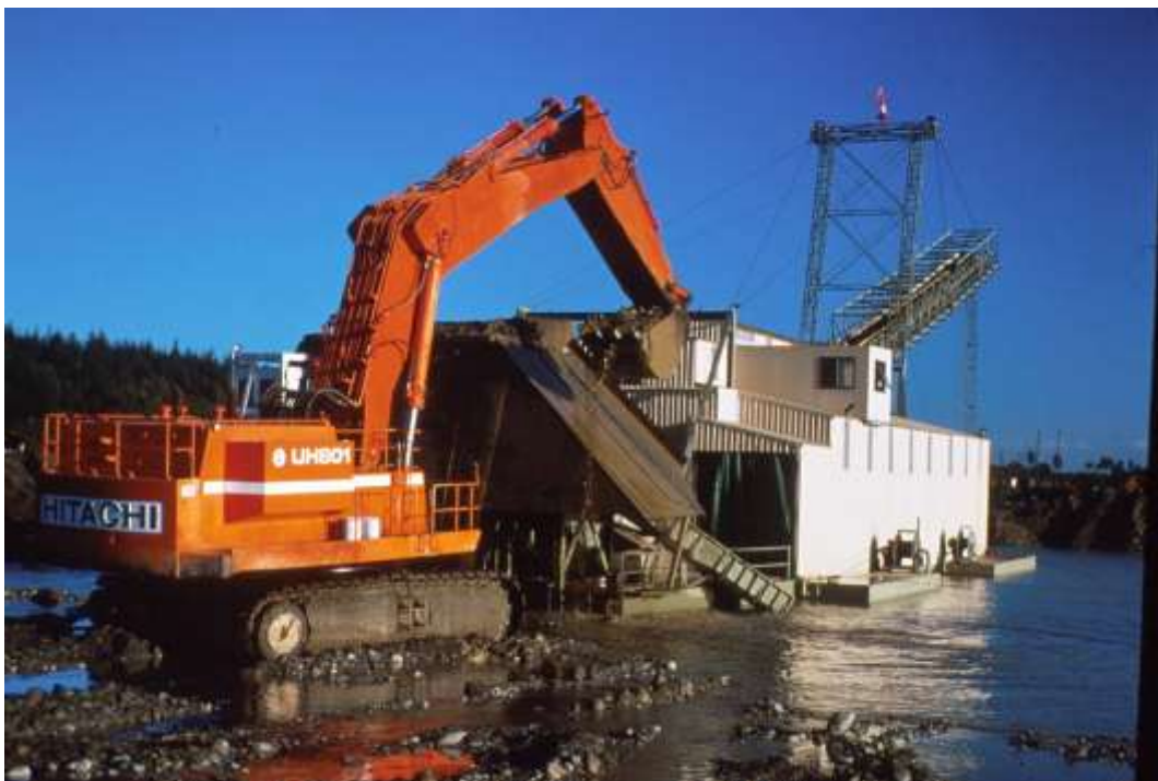
Figure 85 L&M Mining Ltd's No. 6 Plant at Rimu. Gravels 5-22 m thick were fed to the 300 m 3 /hour plant by a 180 tonne hydraulic excavator (photo c. 1995, Eoin Jury).
