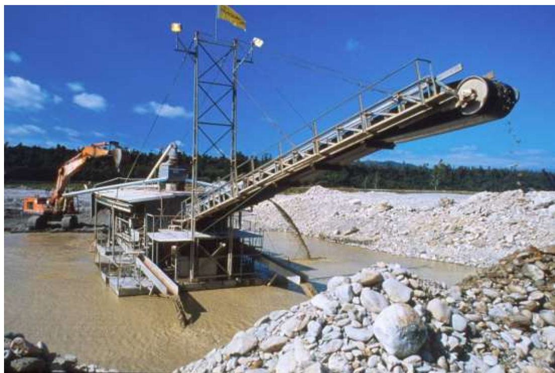
Figure 83 DML Resources alluvial gold plant, Arahura Valley 1995 (Photo Eoin Jury).
