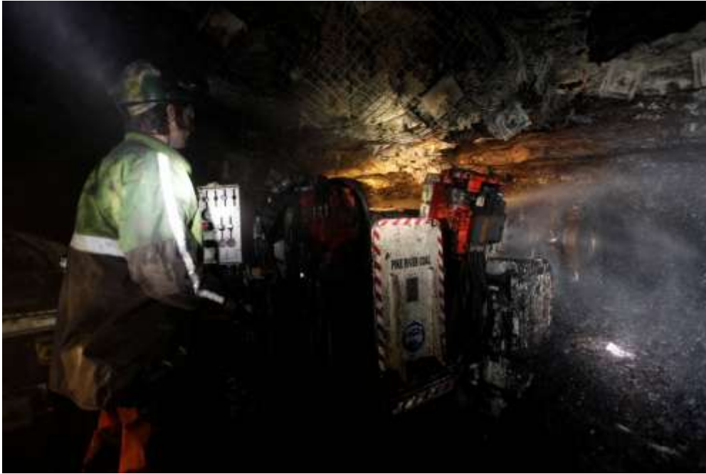
Figure 48 Mining with a continuous miner at Pike River (September 2009 photo courtesy of Pike River Coal Ltd).
