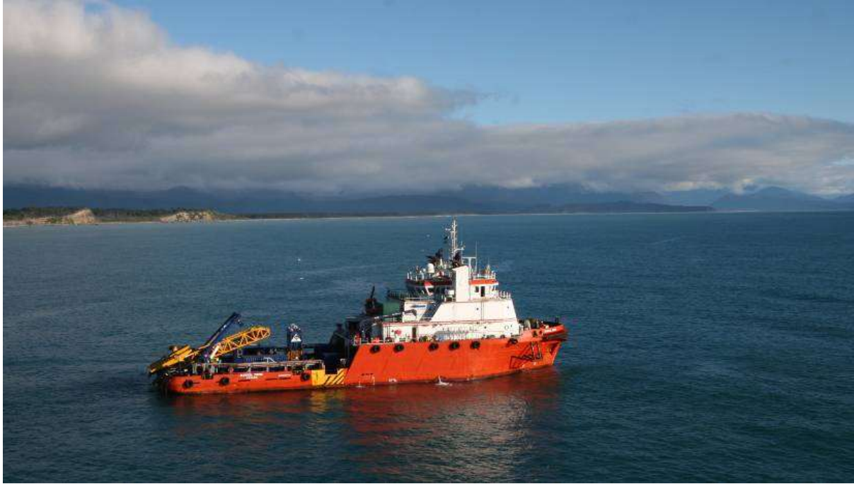
Figure 90 The Marsol Pride, with Seafield Resources core sampling rig raised on the stern, moves to a new drilling site off the West Coast (photo courtesy of Seafield Resources).
