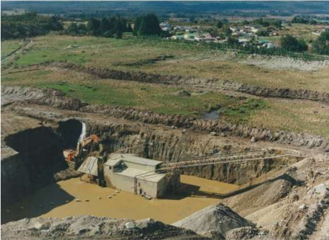
Figure 84 L&M Mining Ltd's Rimu plant fed by a 180 tonne hydraulic excavator (photo after Figure 3 of Manhire et al. 2006).
