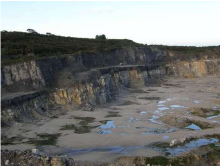
Figure 31 The eastern face of the Cape Foulwind limestone quarry, including the overlying Kaiata Mudstone "marl" that is quarried (photo courtesy Keith Miller, Holcim).
