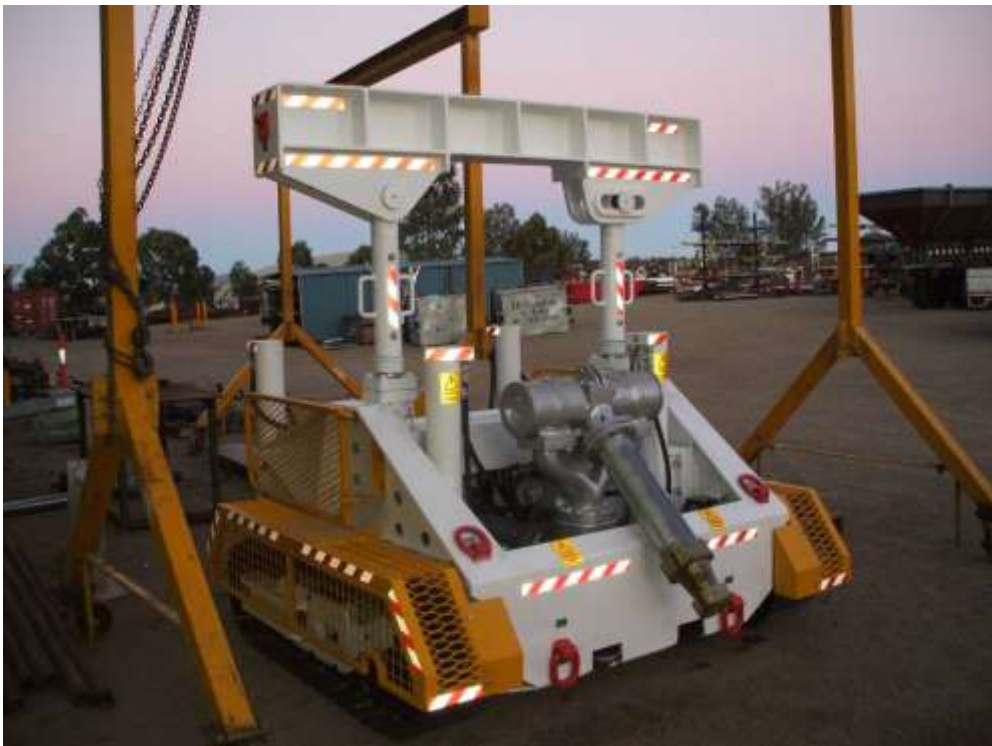
Figure 49 Hydro-monitor used to cut coal using high pressure water, Pike River coal mine (photo courtesy of Pike River Coal Ltd).
