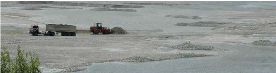
Figure 25 Mining river gravel for aggregate (photo courtesy of Minerals West Coast).
